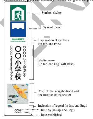
Fig. 12 Shelter guidance type plates
