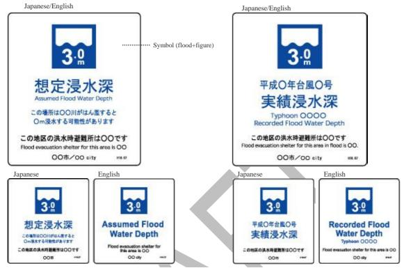
Fig. 6 Flood sign plates (integrated expression with symbols and numbers)
